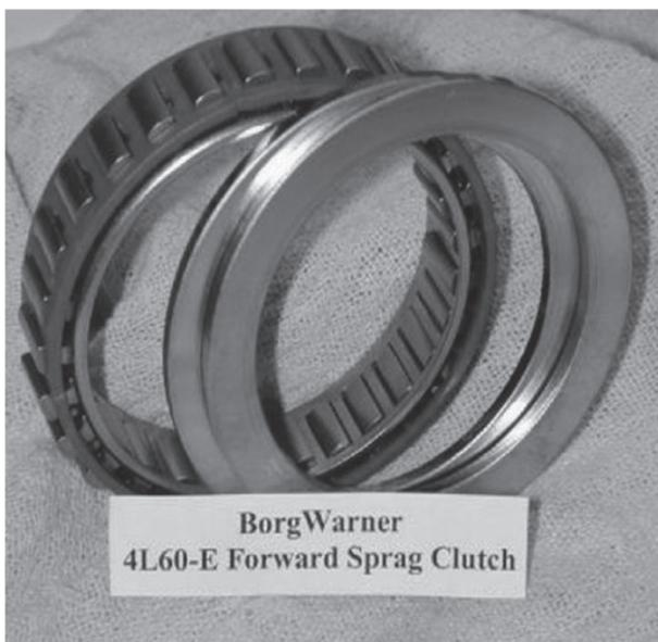
**The Sprag rotates freely clockwise as shown.**
